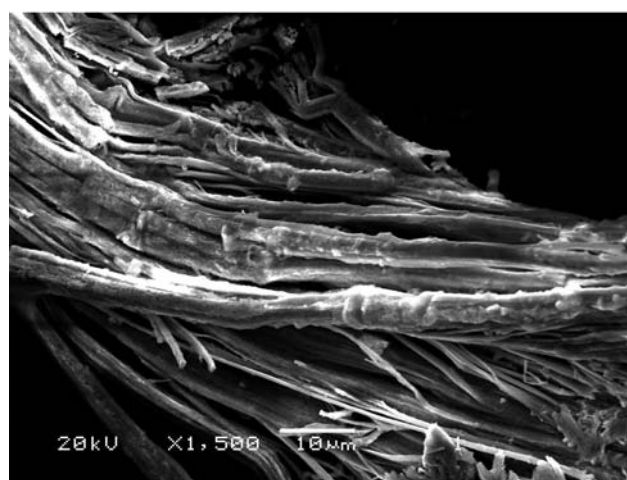
Figure 1. SEM images showing a bundle of fibrous (needle-shaped) crystals of Na 2.8 Cu 5 Sn 5.6 .
